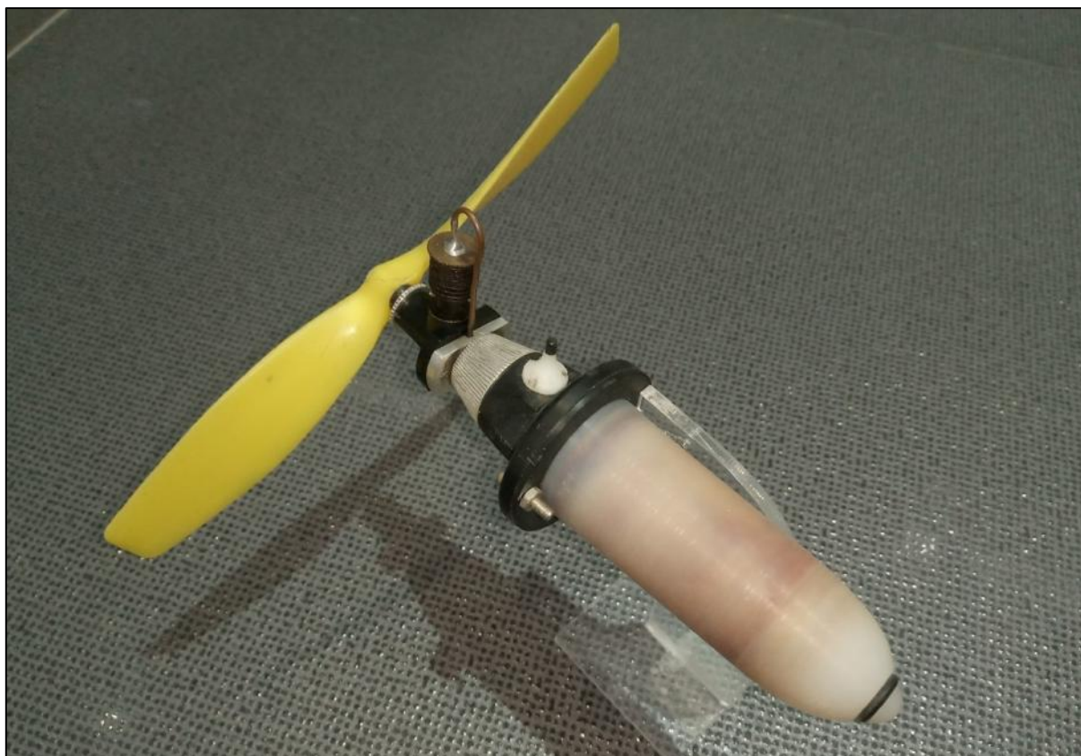
Telco CO_2 motor fitted to Powermaster Mark 5 tank unit
