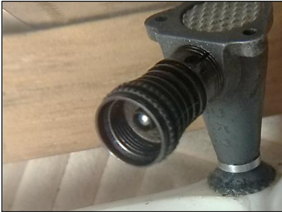
Brown Junior .005 with integral thin steel ball retainer
