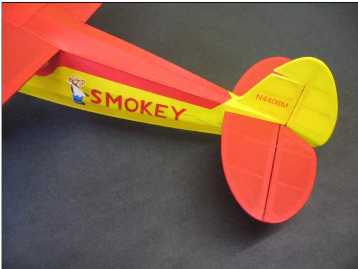
Keil Kraft Junior Flying Scale Piper Super Cruiser converted to three channel radio. Control surfaces are hinged with narrow strips of flexible material cut from a 3.5in floppy disk.
